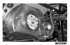
2. Remove the old H4 bulb by unlocking the spring; then insert the new bulb into headlight assembly and lock the spring to secure the bulb.
