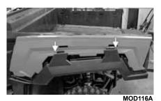
With a suitable pry bar, lift up on the outer cargo box floor near the rear corner.
