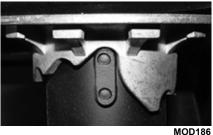
■ NOTE: Before attempting to adjust suspension, clean dirt and debris from the sleeve and remove load from the suspension. Using a suitable lift or jack, lift the vehicle enough to allow the shock assembly to fully extend. Use the spanner wrench to adjust the sleeve to the desired position.
